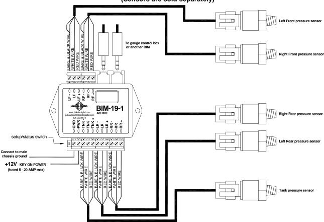
This Bus Interface Module has inputs for up to five solid state pressure sensors. Each input can be configured individually. There are two interface (I/O) ports on the module. Either one can be connected to the gauge system or to another module, allowing several units to be daisy chained together. Do not connect the I/O port to anything other than a Dakota Digital gauge or BIM. Do not mount the module in the engine compartment; it should be mounted in interior of the vehicle.
