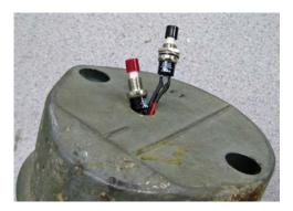
4. Remove the nut and washer from one of the time adjust switches. Pass the one with the nut and washer on through the hole near the center of the can. Pass the other switch through followed by the four individual wires.
