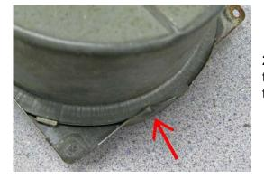
2. Bend open two or three crimps holding the two can halves together and separate them.
