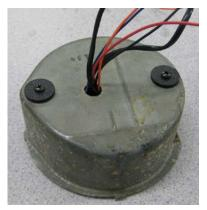
5. Slide the gauge into the can making sure not to pinch the wires when it is fully installed. Through the original light bulb holes install the screws and large plastic washers. Snug but don't fully tighten the screws so alignment can be adjusted.
