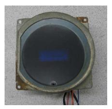
7. Replace the gauge front and re-crimp it to retain it. Install the clock housing to the bezel.
