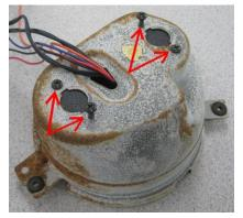
6. Using the 4 included screws provided secure the clock assembly into the housing using the light cover tab holes. It is recommended to start all 4 screws then tighten in a crisscross pattern. Place a bead of silicone around the edge of the opening that the wires pass through to keep them from chaffing.
