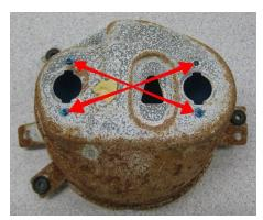
4. From the back of the can cut or grind off the melted plastic tabs that hold in the blue light covers. Remove the light covers.
