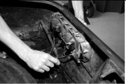
2. Next remove the lens. The lens has tabs locking it into the plastic housing. Pry the tabs gently with a screwdriver to remove lens.
