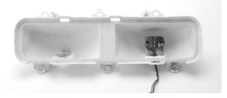
Feed the wires through the larger hole in the mounting plate. Guide the mounting plate to the bottom of the housing. The flat side of the mounting plate should be down and the side with the slight raised center should go up into the housing. This will align the mount in the original housing.
