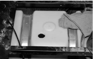
4. Apply fuel resistant sealant to the cork gasket and place gasket on the sensor. The holes of the gasket will only line up with the holes in the sensor in one position so be sure to line up ALL the holes in the gasket with the holes in the sensor.
