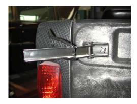
2. Close the tailgate and latch one side. On the side not latched remove the latch wire by pulling it apart as shown. Lift up on the wire pulling it out of the hole and over the back side of the handle. Push it down to remove the bottom side of the wire from the hole and slide it off the end of the handle.
