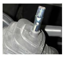
2. Remove the original gear shift knob by pulling up. It helps to twist back and forth as you pull. 3. Insert the new gear shift knob onto the shaft lining up the set screw hole with the hole in the shifter shaft. The set screw will go through the hole and contact the other side of the shifter shaft. Apply thread locker to the set screw. Use a 5/64" Allen wrench to tighten the set screw.
