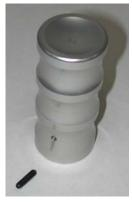
1. Remove the plastic pine tree fastener from the passenger's side of the original gear shift knob. A needle nose pliers works well for this.
