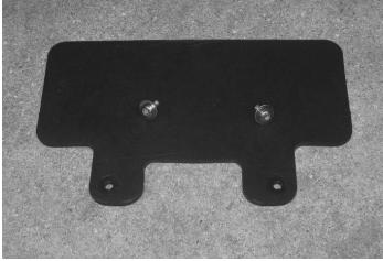
Hold the new Dakota Digital axle guard in place and start one of the bolts through the inner hole along the back edge of the A-Arm. Start a washer and nut to help hold things in place. Do NOT tighten so you have a little flexibility for alignment.
