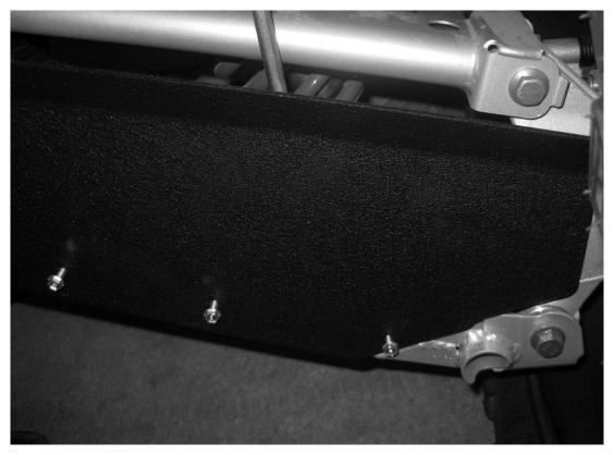
Now go back to the rear of the A-Arm and start the last bolt, watching out for the brake line. Tighten up the hardware on the two bolts to complete the install for this side.
