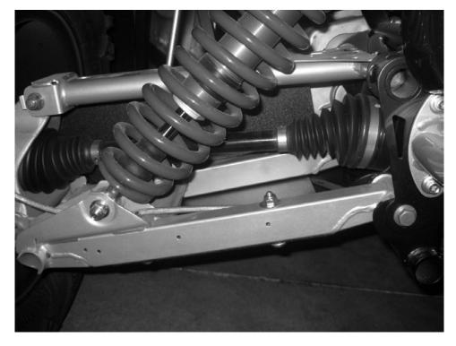
Next, move to the front edge of the A-Arm and hold the axle guard up in place. The three holes in the rock guard should line up with three holes along the front edge of the rear A-Arm. Install three of the self tapping screws here and tighten them up.
