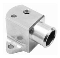
Remove old thermostat housing, saving mounting bolts and the bleed screw. Install the new Dakota Digital housing with hardware removed from factory housing and install any 1/8" NPT thread temp sensor for appropriate water temp gauge.
