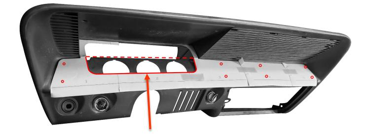
9. Carefully cut out traced section of dash and drill previously marked holes as needed with a size #27 drill bit. If adding an aftermarket radio, cut out the right side as well.
