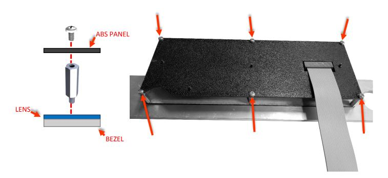
11. Insert the VFD system into the now cut-out dash opening. Secure using the remaining eight screws provided. If a radio will be installed, do so at this time. With a radio installed, you may use only four screws to secure the lens side of the system.
