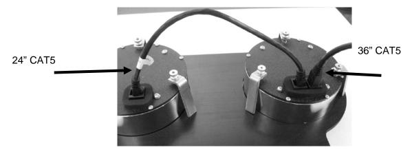
5. System installation is complete. Re-install the dash if you removed it for making holes and refer to the main manual for wiring instructions to complete the VHX installation.
