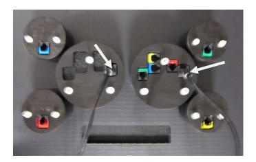
3. Connect the provided CAT5 Cables to the back of the Speed and Tach and carefully route the other ends to the control box mounting location.
