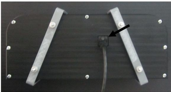
3. Attach the provided CAT5 cable to the back of the VHX display and carefully route the other end to the control box mounting location. Refer to the main manual for wiring instructions.
