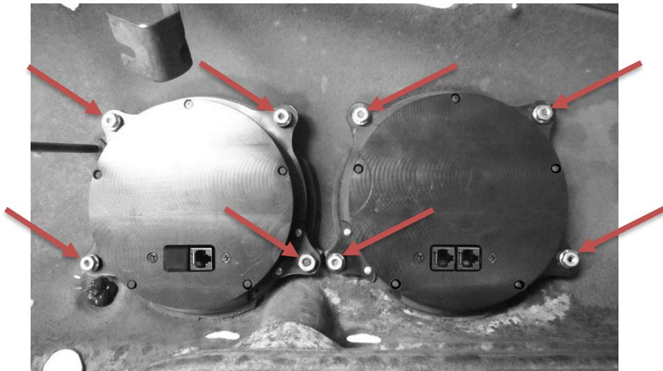
5. Connect the two halves of the new VHX system with the supplied 12" CAT5 cable. Also, route the 36" cable towards the control box location and connect it to the display.
