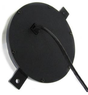
3. Connect the CAT5 cable to the system as the VHX cluster is installed into the dash. Watch carefully so you don't scratch or damage the lens or bezel, and take care when routing the CAT5 cable to the control box location.
