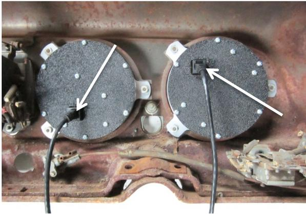
3. Connect a CAT5 cable to the back of each VHX gauges and take care when routing the other ends to the control box mounting location.
