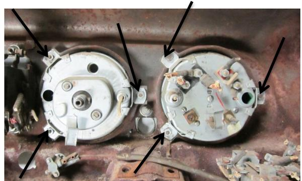
2. The VHX system is a direct replacement of the original cluster, so use the three mounting studs for each gauge along with the factory hardware to secure the VHX system to the dash.
