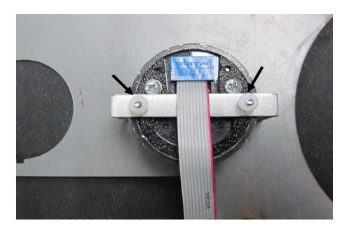
4. Connect the quick disconnect ribbon cables to their respectively labeled counterpart. Note: (OIL-OIL) and (TEMP-TEMP).
