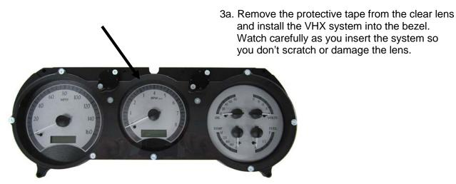
3b. The VHX system should align tightly and the lens should sit flush with the bezel.
