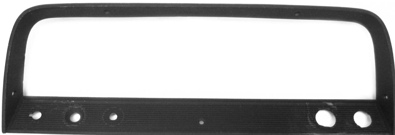
3. Cut the supplied foam tape into six pieces, so each is about two inches long. Stick the foam strips on the angled part of the inside edge of the bezel. The lens will compress against any foam above the edge, which helps prevent lens rattles.
