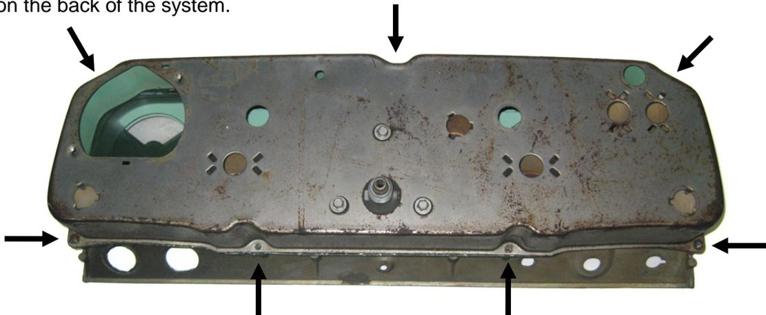
2. Remove the stock gauges, separator plate, and lens from the bezel. The only item to be reused is the original front bezel; the other pieces can be discarded. Now is a good time to clean the bezel and remove any dirt or old lens gasket material.
