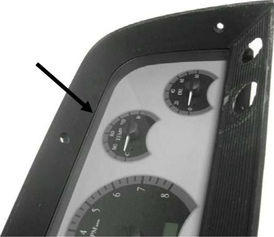
4b. The VHX system should align tightly and the lens should fit flush with the bezel.
