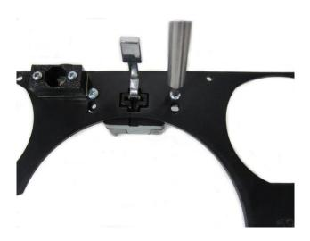
7. Mount the Wiper switch to the ABS plastic panel with the smooth side facing you. The Wiper switch will fit into the large cross hair, and the arm of the switch will slide through the ABS from the rear. Use the provided 3/8" screws with lock washers and nuts to mount the wiper switch to the panel.
