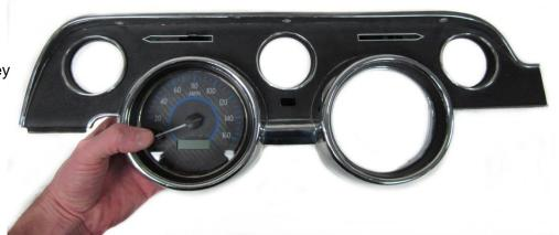
5b. Use the provided 2" screws with lock washers and mount the gauges in place. Do not fully tighten; the holes are slotted to allow minor adjustments to perfectly align each gauge. For the Speedometer and Tachometer, use the two provided brackets at the bottom slots as shown (white arrows). Once aligned, finish tightening the 12 screws using care as to not strip the threads.
