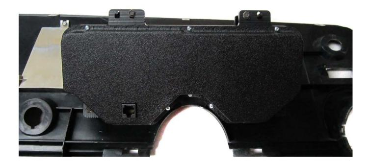
3. Connect the CAT5 cable to the system. As the assembled cluster is installed into the dash, take care when routing this cable to the control box.
