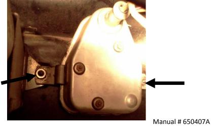
2. With the original clock removed, carefully maneuver the VLK or VLC clock in place from behind the dash while lining up the mounting holes of the clock to the studs behind the dash making sure not to scratch the chrome bezel or clear lens, and then secure the clock in place by using the stock mounting nuts.
