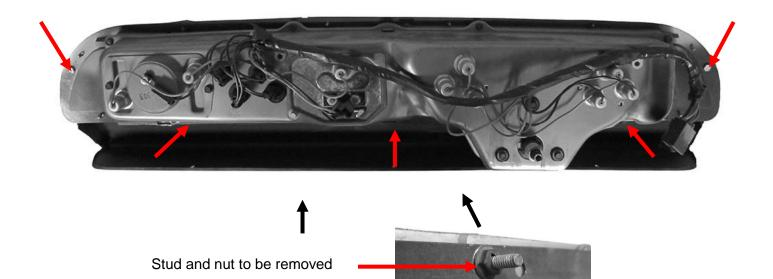
3. Secure the RTX system to the stock bezel using the five stock screws and the provided screw, lock washer, and hex nut in the top center mounting location.
