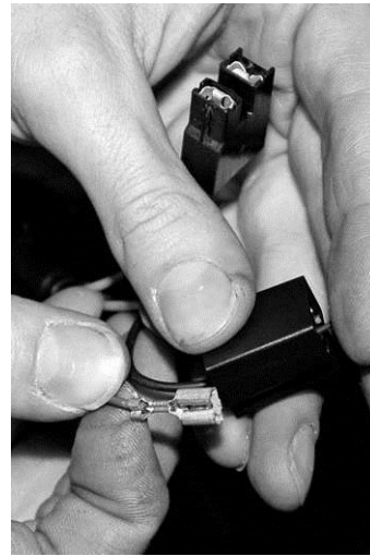
Remove the pin from the connector
