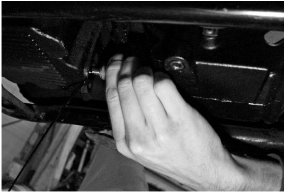
Thread sender into oil pan
