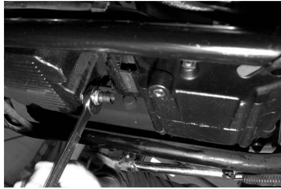
Tighten temp sensor with a 3/4" wrench
