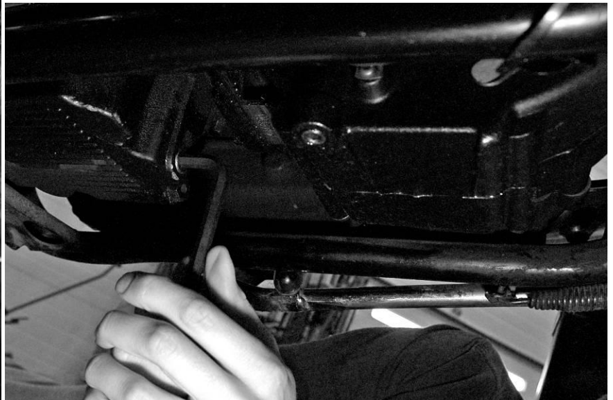
Remove 3/8" NPT allen plug
