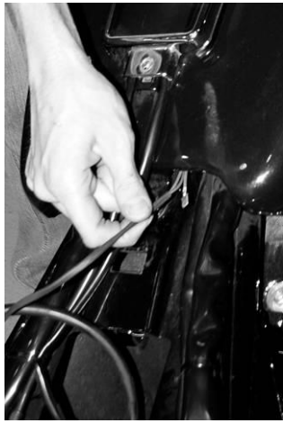
Route wires under tank
