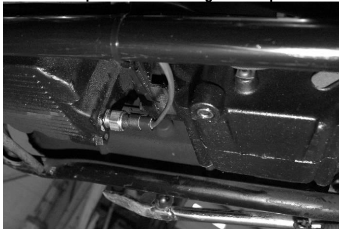
Installed oil temp sensor and harness plug
