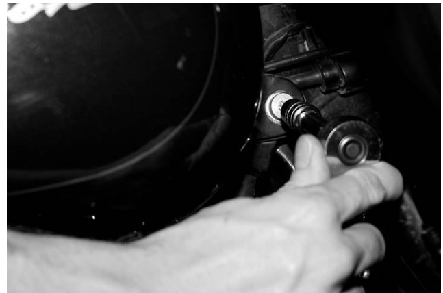
Remove front tank bolts to loosen tank
