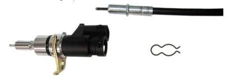
2. Insert the sensor plug in place of the speedometer cable and re-insert the retaining clip to keep it in place.
