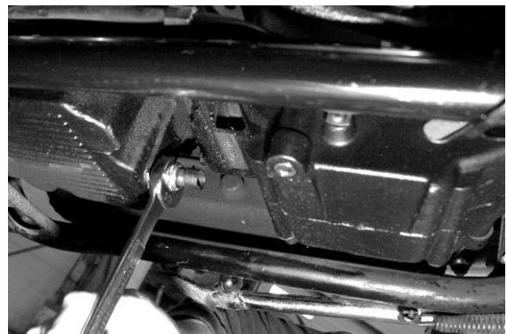
Tighten temp sensor with a 3/4" wrench
