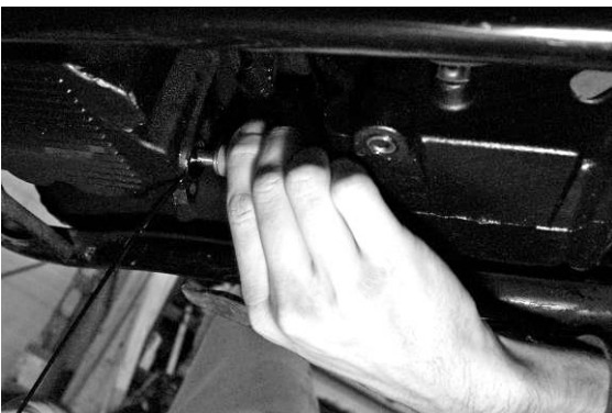
Thread sender into oil pan
