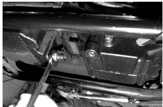
Tighten temp sensor with a 3/4" wrench
