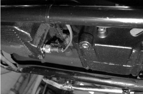
**Installed oil temp sensor and harness plug**
