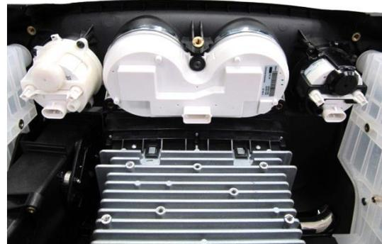
2. Remove the remaining seven (7) screws for removal of the gauges. Ensure the Speed and Tach bezels remain in the fairing.
