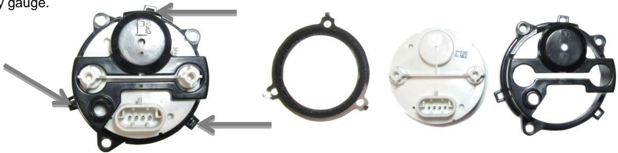
4. The new OIL TEMP gauge will use the existing black Fuel mounting cup and the new VOLTS gauge will use the existing white Volts mounting cup. Place the new VOLTS and OIL TEMP gauges in the appropriate housings and secure the bezel in place by lining up the tabs.
