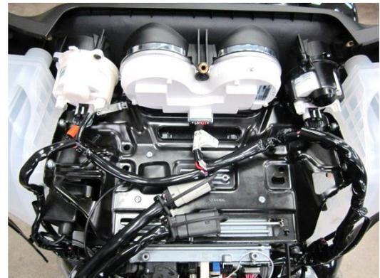
1. Disconnect the three (3) gauges and remove the ten (10) screws securing the amplifier tray to the radio and the speaker enclosures in order to flip the amplifier tray out of the way.
