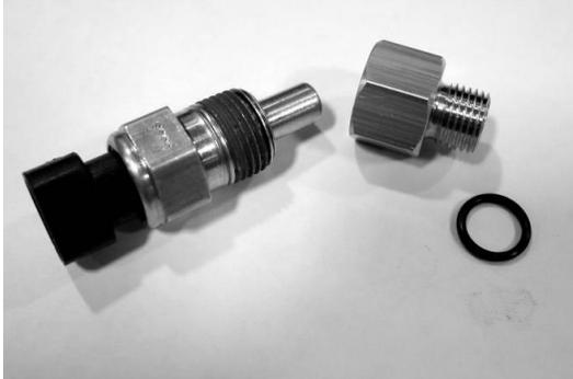
Oil temp sensor, adaptor bushing, and o-ring
