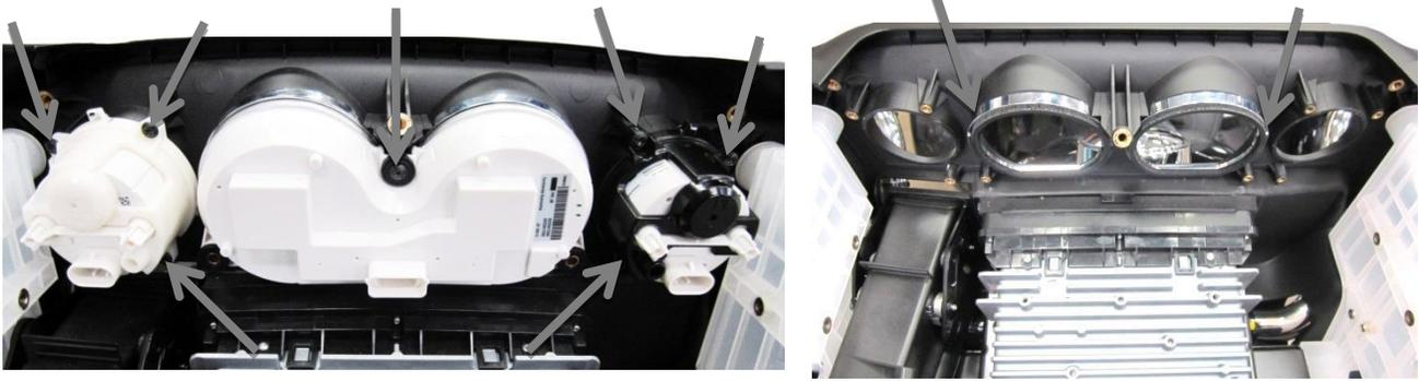
3. The Fuel and Volts bezels and mounting cups will be reused. There are three (3) tabs on the bezels that need to be carefully pushed back through the mounting cup to separate the bezel from the mounting cup and to release the factory gauge.
