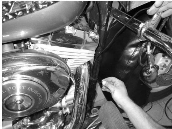
8. You are now ready to make the gauge connections; the Speed/Tach uses the factory Speed/Tach connector, the Volts and Oil Temp use the two (2) provided interconnect harnesses with one end connected to each gauge and the other ends going to either top or bottom connectors on the Speed/Tach. The stock Fuel and Volts connector can be held aside using provided zip ties.
