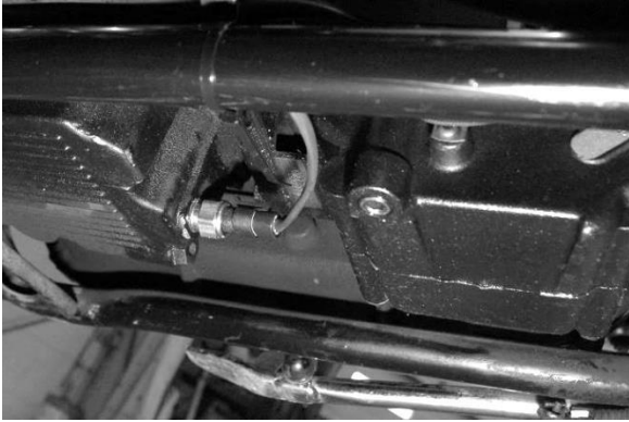
Installed oil temp sensor and harness plug
