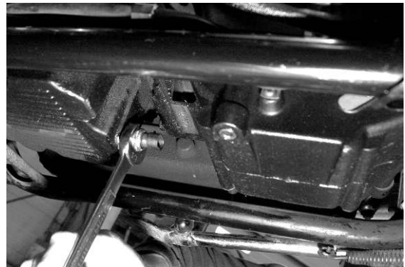
Tighten temp sensor with a 3/4" wrench
