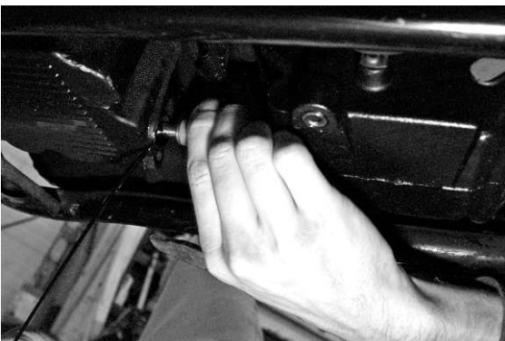
Thread sender into oil pan
