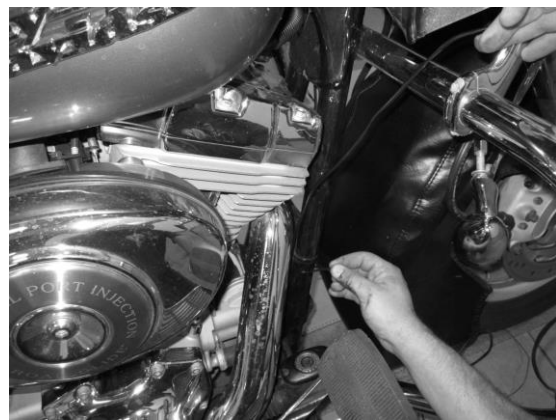
Tighten temp sensor with a 3/4" wrench
