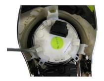
Insure that the rubber gasket is still in the dash or remove from factory gauge and place back on dash
