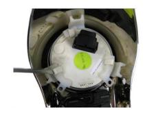
Remove the rubber gasket from the factory gauge bezel.
