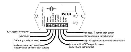
If the NORMAL output does not drive your tachometer, use HI VOLT.
