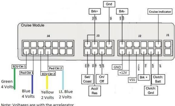
Note: Voltages are with the accelerator pedal fully pressed to the floor. Ensure the key is in the 'on' position and the engine is NOT running.
