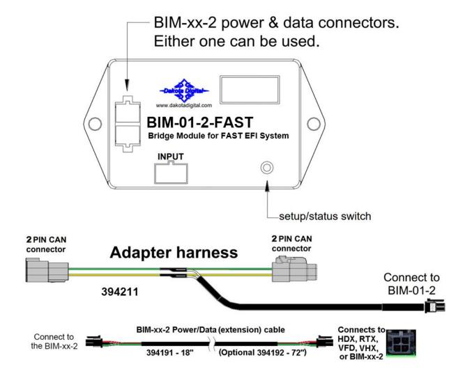
This Bus Interface Module is designed to read engine information from FAST XFI and EZ-EFI 2.0 systems as well as TCI EZ-TCU kits. FAST EZ-EFI kits are <u>not</u> compatible. This module is connected to the FAST/TCI kits through the included Y-adapter harness. This can be plugged in line with the dedicated CAN terminals on the EFI/TCU harness.
