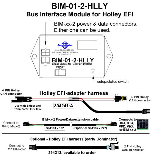
This Bus Interface Module is designed to read engine information from specific Holley EFI kits. The Holley Terminator, HP, Sniper, Dominator and Terminator X and X Max. The module is connected to the Holley EFI through the CAN-bus plug on the EFI harness. Depending on your EFI module you may have a 2-pin or 4-pin CAN connector. We supply EFI adapter harnesses that will allow you to connect with your particular kit.
