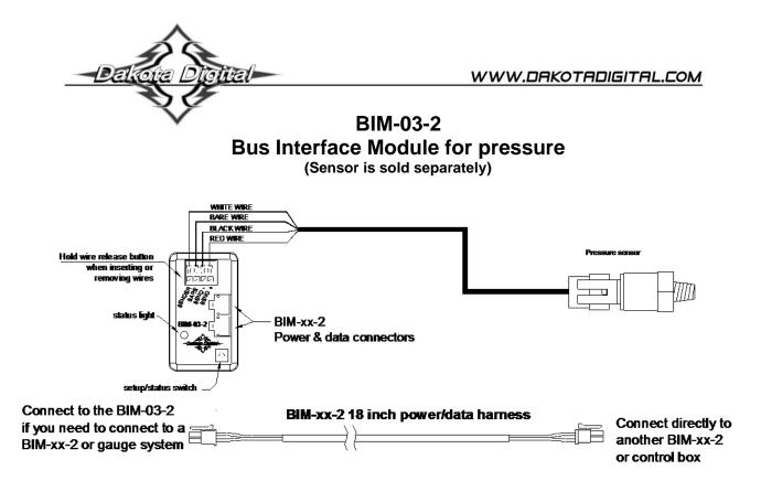
This Bus Interface Module connects to a solid state pressure sensor. There are two power & data interface (I/O) ports on the module. Either one can be connected to the gauge system or to another module, allowing several units to be daisy chained together. Do not connect the I/O port to anything other than a Dakota Digital gauge or BIM. Do not mount the module in the engine compartment; it should be mounted in interior of the vehicle.
