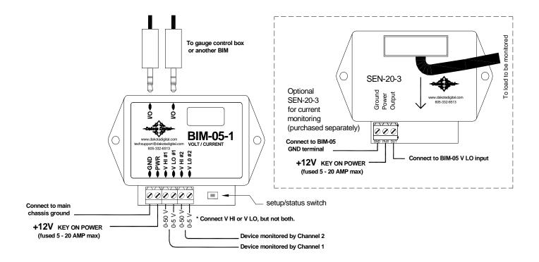
This Bus Interface Module has inputs for up to two devices to be monitored. Each channel can be configured individually. There are two interface (I/O) ports on the module. Either one can be connected to the gauge system or to another module, allowing several units to be daisy chained together. Do not connect the I/O port to anything other than a Dakota Digital gauge or BIM. Do not mount the module in the engine compartment; it should be mounted in interior of the vehicle.
