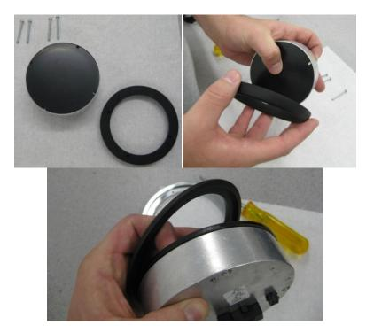
Start one screw a couple turns, do not fully tighten. Use care when aligning the bezel to avoid scratching the lens. Pivoting off the started screw as needed, start the remaining three screws. Tighten up the remaining screws in a criss-cross pattern, approximately 5.5 in-lbs of torque. DO NOT over tighten!
