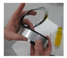
Locate the black bezel and four, 4-40 x 1.25" screws. While holding the gauge housing and lens, install one of the screws from the back of the housing and up through the lens; hold the screw in place with your finger. Carefully align this screw with one of the holes in the bezel to get started.
