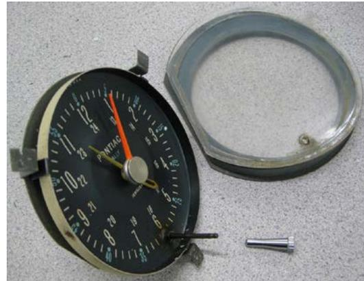
3. Remove the knob from the clock shaft. Hold the gear on the back while unscrewing the knob. If it does not unscrew you will need to cut the shaft.
