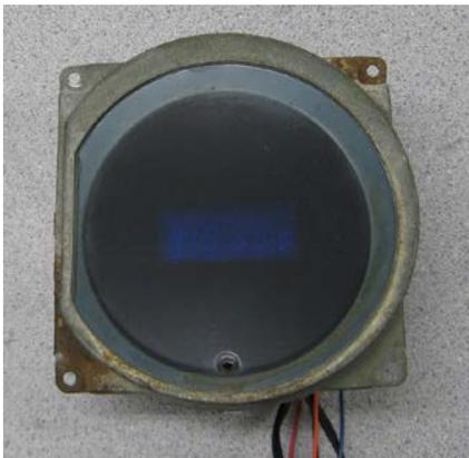
7. Replace the gauge front and re-crimp it to retain it. Install the clock housing to the bezel.
