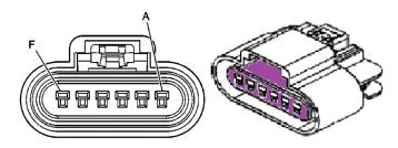
The GM throttle pins are labeled A through F.
