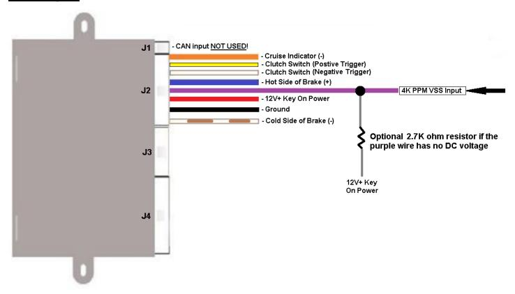
All Dakota Digital control boxes, (and the GPS-50-2 CRUISE terminal), will need the pull up resistor added, as long as the control box is being fed a speed signal into the speed input wires.
