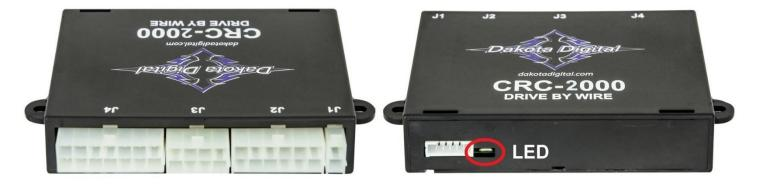
The small connector in the back is not used, but there is a small cutaway for an LED, that can used to observe operation and limited diagnostics, (see page [12]).
