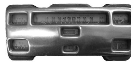
2. From the rear of the dash; insert the HDX system into the opening and securely mount using the stock hardware from disassembly
