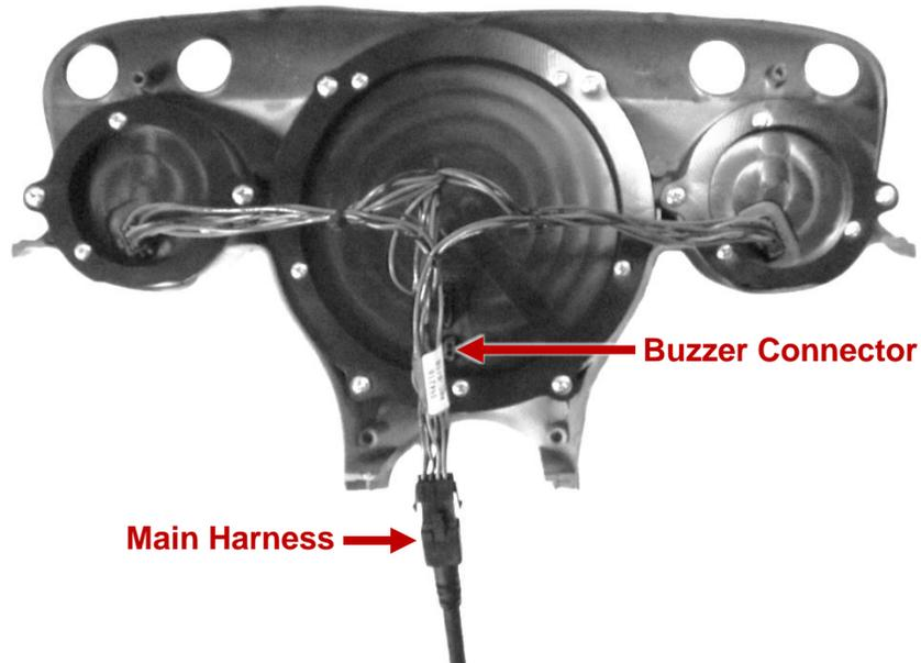
6. Re-install the cluster into the vehicle using the retained factory hardware. Refer to the main HDX manual for wiring instructions to complete the installation.
