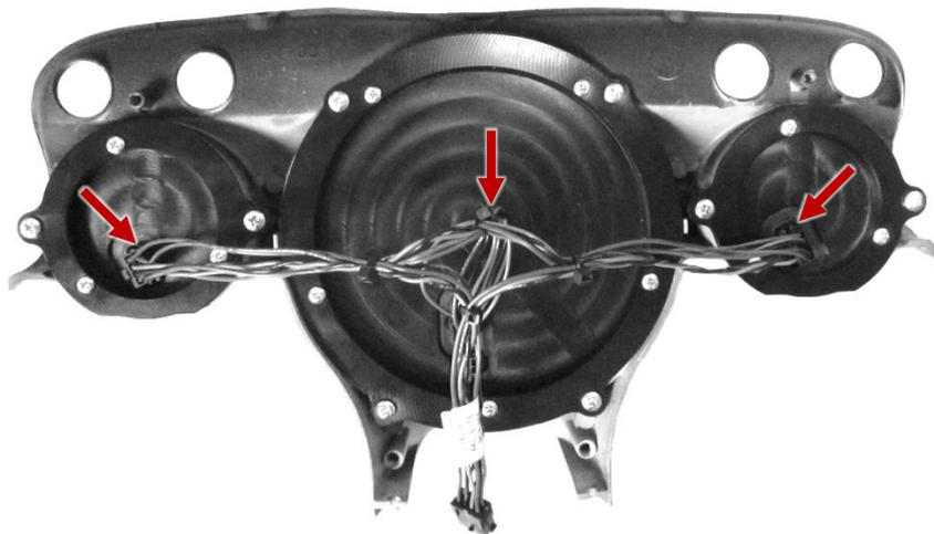
5. Connect the provided main harness to the interconnect harness. The buzzer (optional, for audio feedback) may also be connected to the back of the HDX system. Carefully route the other ends of these harnesses to the control box and buzzer mounting locations respectively.
