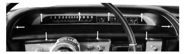
2. Separate the stock gauges from the bezel by removing the five screws securing the gauges to the bezel. There is also a nut to remove from a stud on the top side of the gauges. The five screws will be re-used for reassembly.
