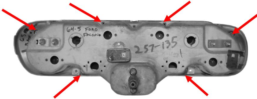
3. With the bare bezel lying face down, fit the HDX system into place and secure it to the bezel using six original screws from disassembly.
