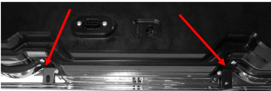
5. Connect the provided harness and the buzzer (optional for audio feedback) to the back of the HDX system.
