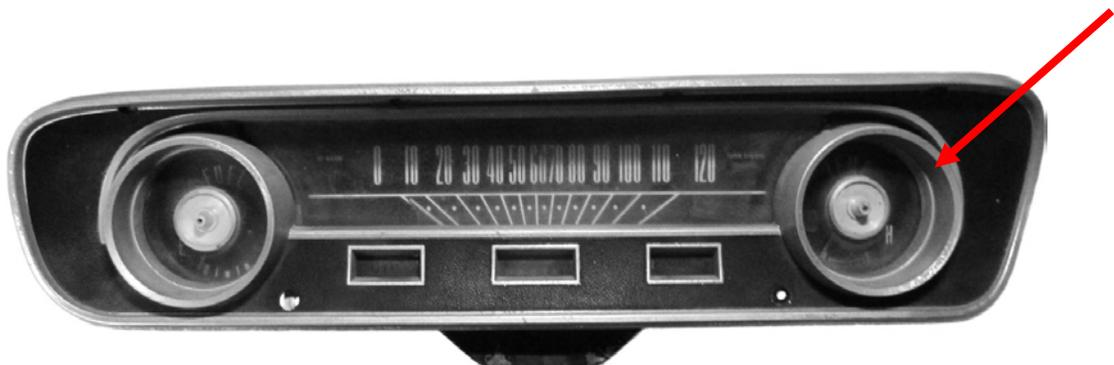
2. Separate the bezel from the rest of the cluster by removing the seven screws on the backside. Retain six of these screws for reassembly.
