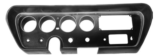
2. Remove the stock gauges, separator plate, and lens from the bezel. The only item to be reused is the original front bezel; the other pieces can be discarded. Now is a good time to clean or refinish the bezel.
