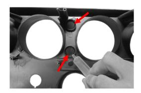
4. Place the HDX system into the bezel, taking care to align all mounting holes. Secure the three (3) provided countersunk screws on the bottom mounting points; move to the top and secure the three (3) pan head screws.
