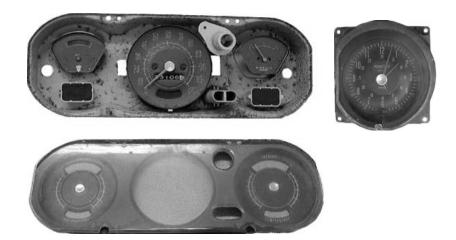
3. Peel the paper off the two block off lenses that match the bezel and, on the back of the housing, place them shiny side down in the two indicator openings in the center. Use silicone to hold them in place and avoid handling until the block off lenses are secure.
