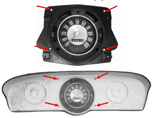
3. The only part that will be re-used is the stamped bezel and the screws that mount the bezel.
