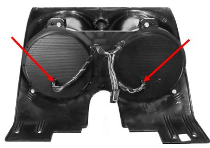
6. Connect the provided interconnect harness to the back of the HDX system.
