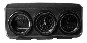
9. Remove the console gauge assembly from the console.
