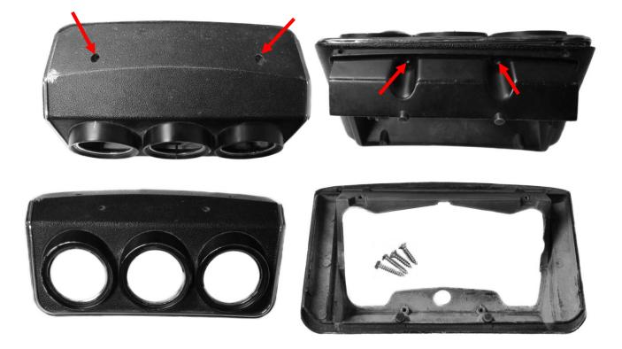
11. With the top half of the housing face down; place the gauge system so they are aligned appropriately inside the housing. Note: the two bosses on the top portion of the housing will align to the two notches in the HDX system. Cut the remaining pieces of foam tape into 1" pieces and place over the back of the HDX console cluster tabs. Be sure not to cover the holes for mounting the back plate.
