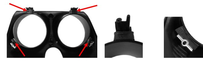
On the top two locations, fold the foam over the edges and make sure it's not sticking into the visible window. In the bottom two corners, the area for the tape is slightly narrower than the foam so you will need to ensure the foam is curved with the opening in the housing.
