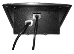
14. Connect the clock harness and the other main harness to the back of the assembled cluster and carefully route the other ends to the Control Box mounting location. 15. Connect the provided Y harness to the Control Box so both main harnesses can be connected.
