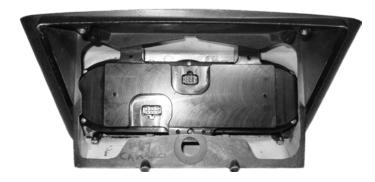
12. Align the bottom portion of the console housing over the back of the VHX console system and mount the two halves of the housing back together with the factory screws.
