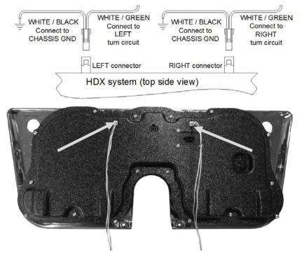
5. Connect the provided main harness, clock harness, and the buzzer (optional for audio feedback) to the back of the HDX system.
