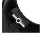
On the top two locations, fold the foam over the edges and make sure it's not sticking into the visible window. In the bottom two corners, the area for the tape is slightly narrower than the foam so you will need to ensure the foam is curved with the opening in the housing.
