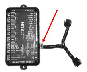
14. Carefully route both main harnesses to the control box mounting location and connect to the Y harness; refer to the main manual for wiring instructions to complete the HDX installation.
