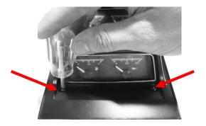
12. With the bezel mounted to the HDX system, align the cluster back into the console and use the provided four (4) fender washers and thumb nuts provided to secure the cluster to the console. Also connect the final main harness to the back of the HDX system. The console is now ready to reinstall back into the vehicle.
