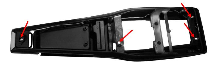
10. Remove the gauge cluster from the console by removing the four (4) screws holding the cluster to the console. Also remove the top screws that hold the bezel to the housing as shown in the picture. The bezel and screws will be reused for the new gauges.
