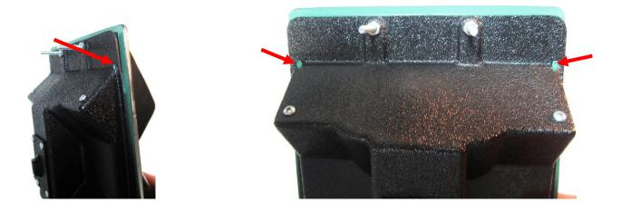
11b. Attach the bezel to the HDX cluster using the original screws from disassembly and the two (2) flat spring nuts provided.
