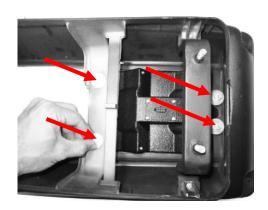
Route cable between the HDX system and bracket NOT UNDER THE BRACKET
