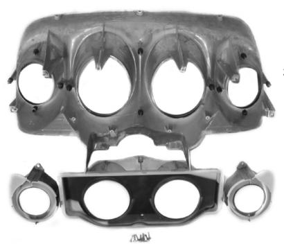
2. Remove the stock gauge cluster from the bezel and save the three separator pieces and the hardware for reassembly.
