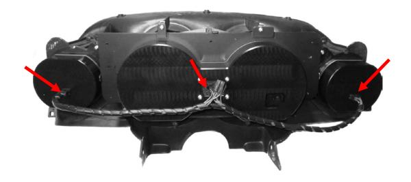
6. Connect the provided main harness and the buzzer (optional for audio feedback) to the back of the HDX system.
