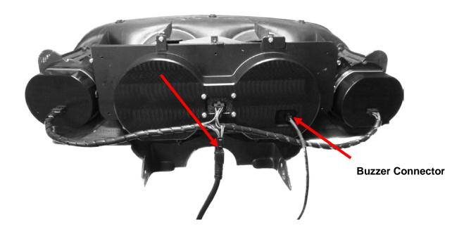
7. Re-install the cluster into the vehicle using the factory hardware and refer to the main manual for wiring instructions to complete the HDX installation.
