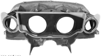
4. Align the HDX system on the separator pieces and use the stock hardware to secure to the bezel. The bottom two mounts of the Speed and Tach assembly will use the supplied 3/4" counter sunk screws as shown with the blue arrows.
