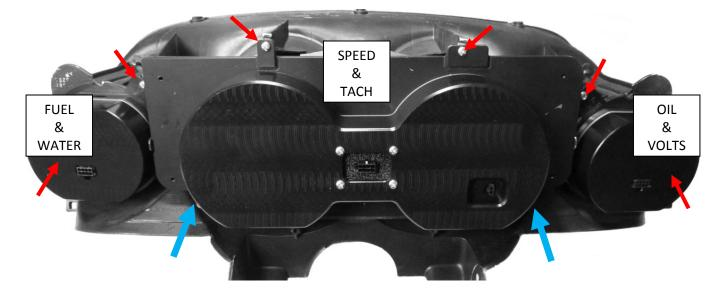
5. Make the interconnect harness connections to the gauges with their respective length ends.
